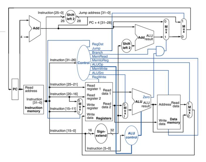
The register file will produce two values along the read data 1 and read data 2 buses. Read data 1 is always sent to the Arithmetic Logic Unit (ALU).
