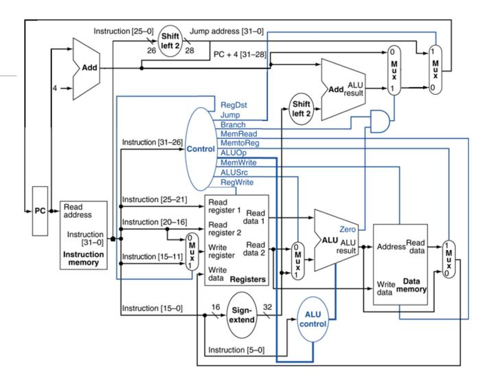
The next five bits [bits 25-21] are sent to the register file to identify the first register we will be reading from. We always do this, even if the instruction does not need to read any registers.
