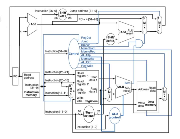
All of the decisions to be made on the datapath are controlled by multiplexors and control signals (shown in blue).
