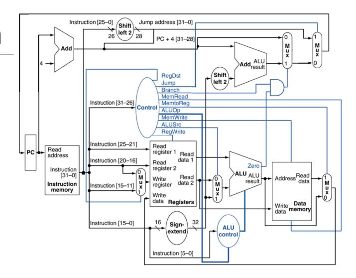
In a BEQ instruction, we calculate a branch target address by shifting our sign-extended immediate to the left twice. This is the same as multiplying it by four.
