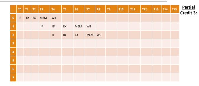
In instruction two, we are trying to add \$t0 and \$s0 together. Neither of these registers have been modified by our segment of assembly code, so this instruction should be able to proceed without a hazard.
