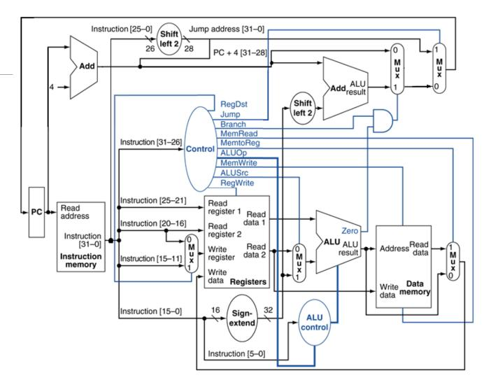
The ALU will produce a result based on the inputs provided and the ALU operation signal from the ALU control unit.
