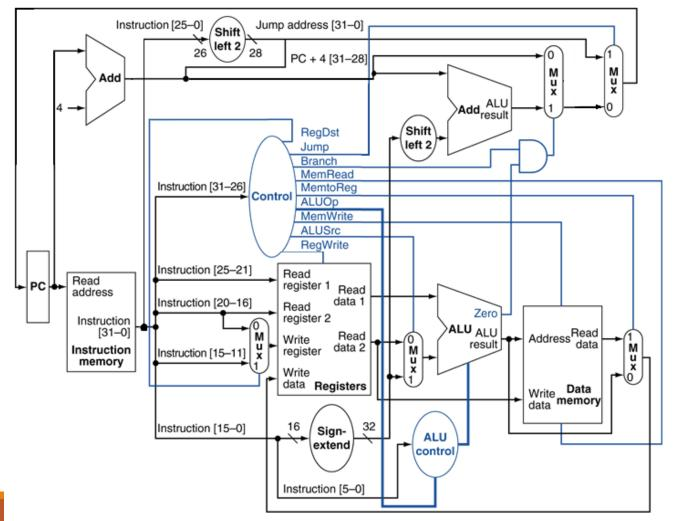
RegWrite gives the processor permission to write to the register file.
