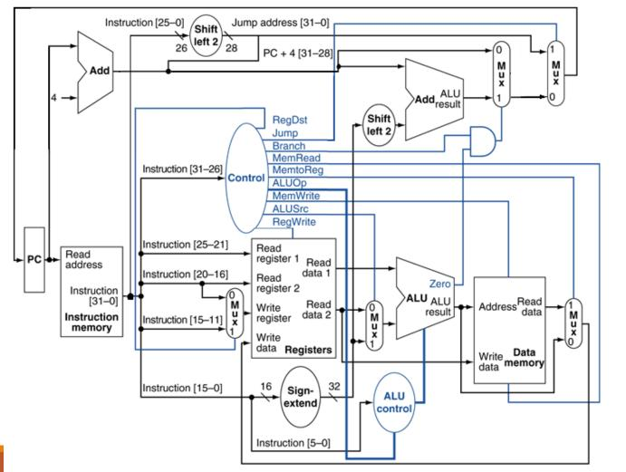
MemtoReg determines which result we are going to send back to the register file.
