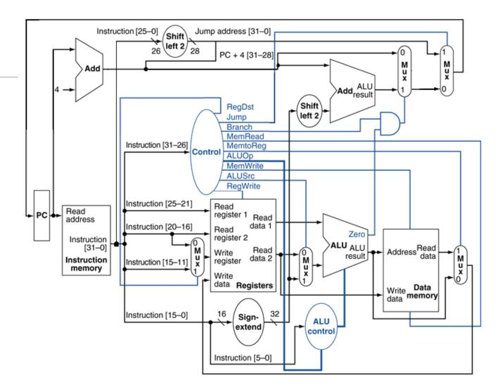
In a lw instruction, we take a value out of memory and send it back to the register. This creates two possible values for write data. We use a multiplexor to choose between ALU result and read data.
