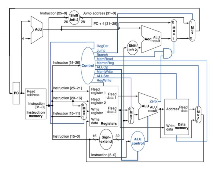
The next five bits [bits 15-11] are sent to the write register multiplexor. In R-Type instructions, this will be the register that receives a new value.
