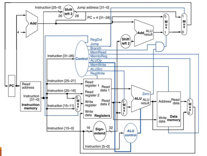
The Control Unit sets all the control signals based on the Opcode.
