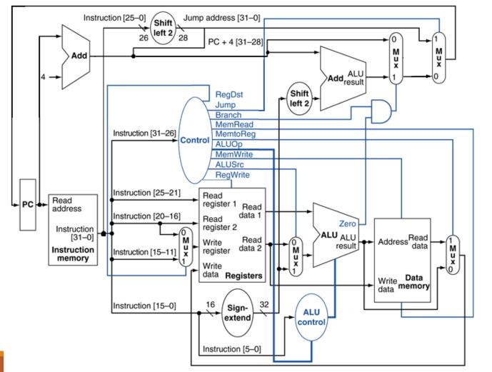
ALUSrc stands for ALU source. This determines the second input for the Arithmetic Logic Unit. It has to choose between read data 2 and the signextended immediate value.
