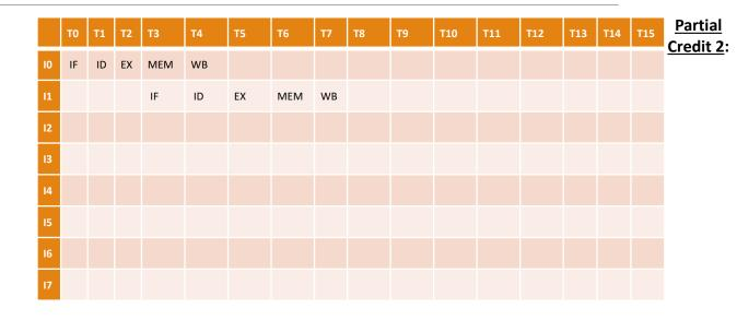
In instruction one, we are trying to add \$t4 and \$s2 together. However, \$t4 is being written by the previous instruction – instruction zero. In the chart we can see that this value does not reach the register file until T4. Since we write in the first half of the clock cycle and read in the second, we can overlap the WB stage of I0 and the ID stage of I1.
