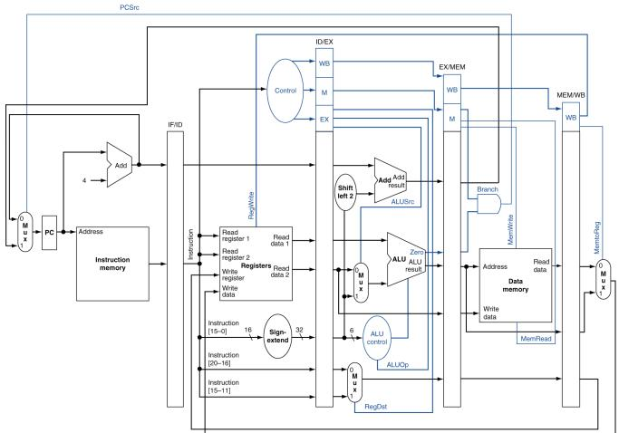
Similar to data hazards, the easiest method is to stall until the branch has been resolved.
