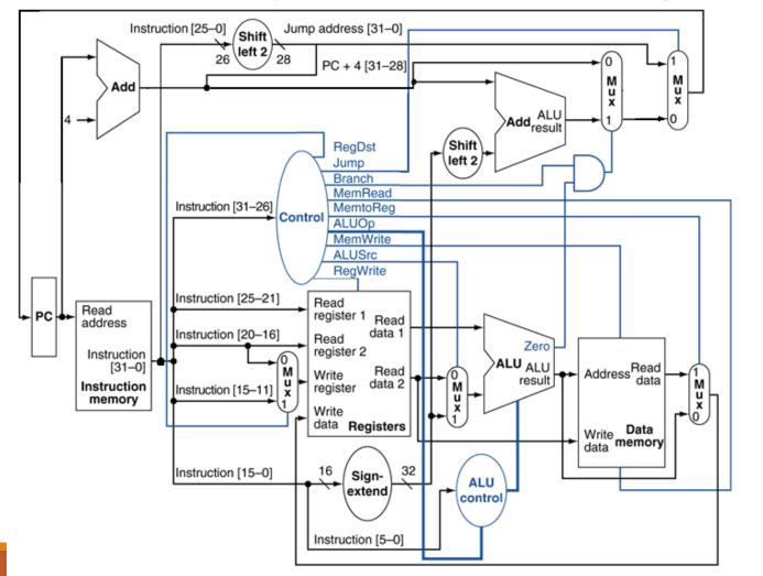
How should the control signals be set for an addi instruction?
