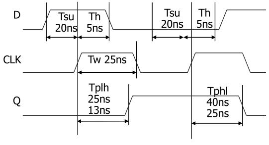
all measurements are made from the clocking event: the rising edge of the clock
