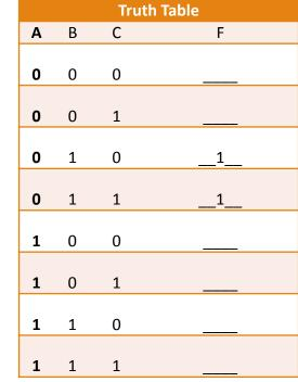
Complete a truth table that has 3 inputs (A, B, and C) and one output (F). F is asserted whenever Given: B is asserted but A is not. F is also asserted whenever C is asserted. F is deasserted in all other cases.
