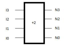
Design a combinational hardware element that counts even numbers. The system must be given a non-negative even number as input and will return as output the next even number. For example, when given the number 2 the system will output the number 4. All numbers will be in binary. The largest number the system can accept is 14, but it will return 0 in this case. When the system is given an odd number, it will also return 0.
