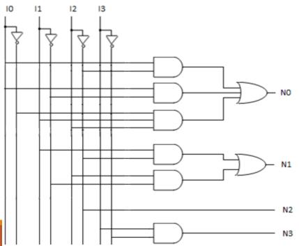
Design a combinational hardware element that counts even numbers. The system must be given a non-negative even number as input and will return as output the next even number. For example, when given the number 2 the system will output the number 4. All numbers will be in binary. The largest number the system can accept is 14, but it will return 0 in this case. When the system is given an odd number, it will also return 0.
