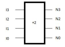
Design a combinational hardware element that counts even numbers. The system must be given a non-negative even number as input and will return as output the next even number. For example, when given the number 2 the system will output the number 4. All numbers will be in binary. The largest number the system can accept is 14, but it will return 0 in this case. The system cannot be given odd numbers; assume this is verified before the inputs are given to the system.
